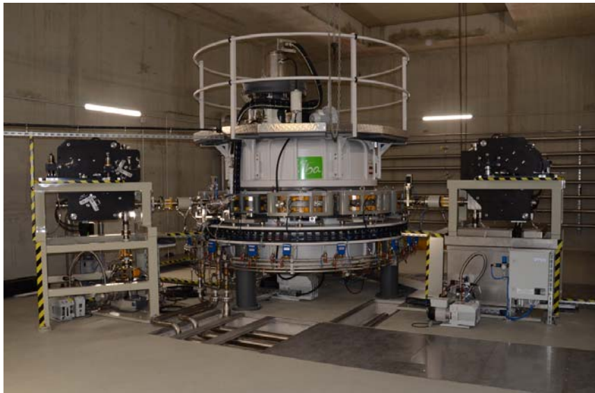
190 kW Power E-Beam: 10 MeV 19 mA
